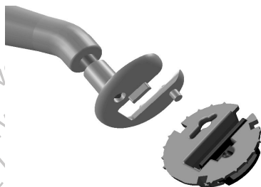
Figure 19. Attach Retaining Clip to Horseshoe End of Tool
