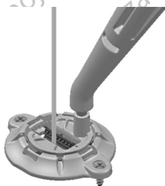
Figure 20. Position the Retaining Clip Over the Base
