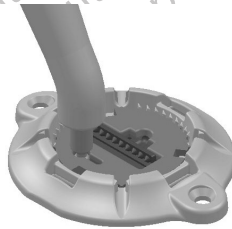
Figure 41. Inserting the Placement/Removal Tool
