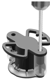
Figure 8. Base Attached to the Butterfly Holding Tool with Screwdriver Inserted
