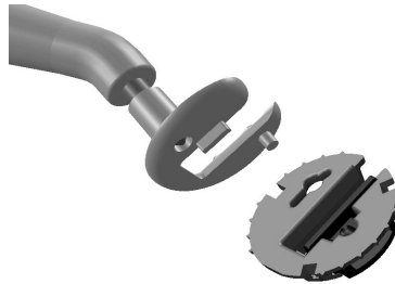
Figure 20. Attach Retaining Clip to Horseshoe End of Tool
