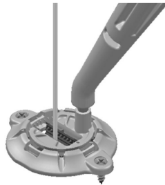
Figure 21. Position the Retaining Clip Over the Base
