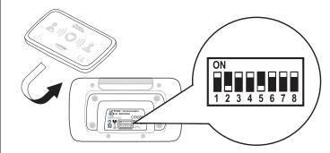
Check the white switches numbered 1-8 on the bottom of your Communicator. If they match the switch settings shown above, no action is needed. If they do not match, slide them up or down to set them as shown.
