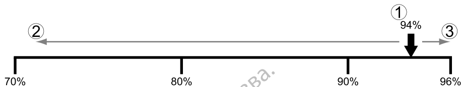
[1] Nominal RhythmMatch Threshold value [2] Less sensitive to VT, more specific for SVT [3] More sensitive to VT, less specific for SVT
