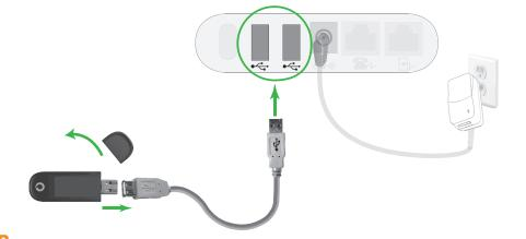
B. Internet Connection, using a USB Ethernet Adapter
