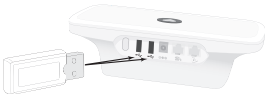
Figure 9. Connecting a USB Accessory Adapter
