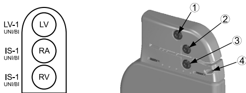
Figure 5. Lead connections and setscrew locations, RA: IS-1, RV: IS-1, LV: IS-1
