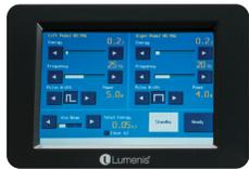
The graphical user interface with a touch screen allows for the tracking of accumulated energy during the procedure and double settings are controlled by the systems' dual pedals.
