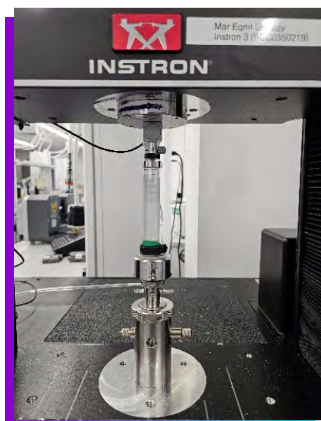
Figure 1. Sample set up under the universal testing machine. The compression plate on the machine moved down, applying a force onto the plunger. This transferred that force onto the hydrogel sample placed at the bottom of the cylinder. Changes in plunger height were recorded and later used to calculate change in sample volume.
