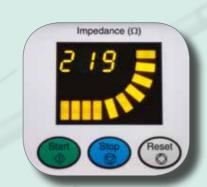
Impedance rise is indicated by an increase in ohms  $(\Omega)$  and a sequential illumination of the bars on the front panel, signaling cellular destruction and the completion of a thermal lesion.
