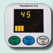
Initial tissue impedance is measured prior to application and is typically within the range of 40 to 80 ohms  $(\Omega)$ , illumination three bars on the front panel of the RF 3000 Generator
