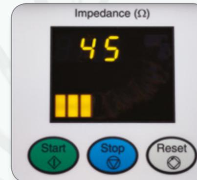
Initial tissue impedance is measured prior to application and is typically within the range of 40 to 80 ohms ( $\Omega$ ), illumination three bars on the front panel of the RF 3000 Generator.
