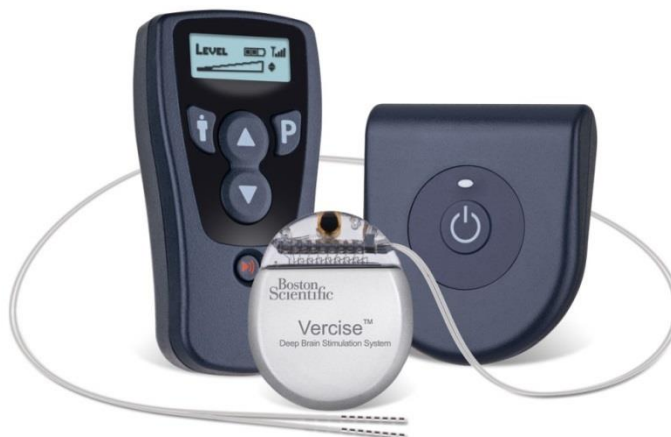
From left to right: the Vercise Deep Brain Stimulation System consists of a remote control, stimulator with attached leads, and charger.
