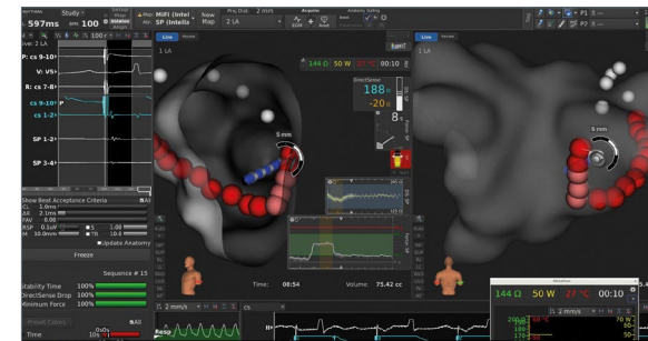
Figure 3. The role of the tip widget and tag coloring are shown. Before RF is initiated, we aim for a CF value between 10-44g (displayed in the force graph). The catheter widget displays 4/6 blocks in green. RF delivery is tailored to the LI drop. For the posterior wall, 10 seconds or maximum LI drop of 15 ohms, whichever comes first. For the anterior wall, 20 seconds or a maximum LI drop of 30 ohms, whichever comes first. Tag coloring ranges from dark pink >15 ohms and red >25 ohms. Pale pink ablation tags display <15 ohm drop in Local Impedance and quickly identify 'weak links' in RF ablation application.
