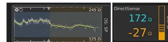
Figure 7a. Example of Local Impedance drop during RF application.
