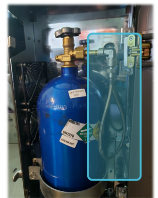
Appropriate console tank hose looping
