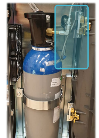
Inappropriate console tank hose looping may exert additional weight on the tank scale
