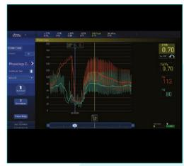
smFFR automatically excludes certain artifacts (e.g., flushing, opening AO stopcock or hemostasis valve, pulling out guidewire during recording) to latch to the true FFR value.
