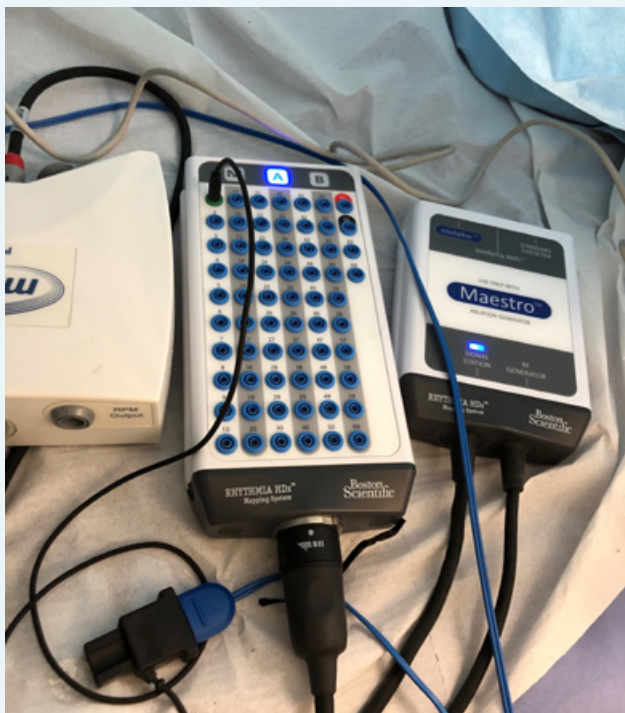
Figure 3: Connection of RF back patch used as system reference to PIN A1 via INTELLATIP MiFi™ filter cable
