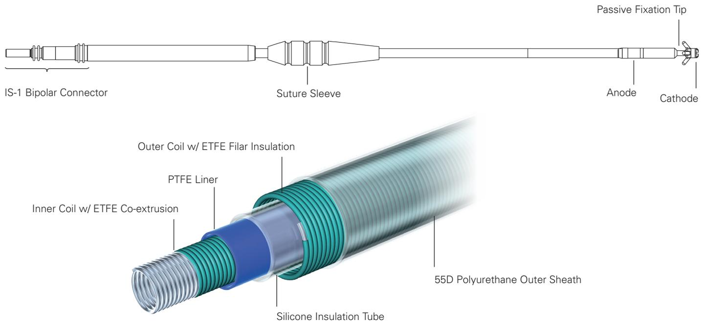
**IROX™-coated Electrodes:** The electrodes are coated with IROX to increase the microscopic surface area.
