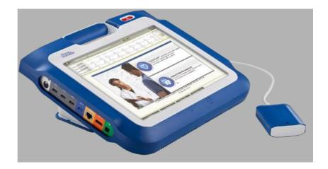
The LATITUDE Programming System, Model 3300 is a portable cardiac rhythm management (CRM) programming system designed to allow health care providers to interrogate, monitor and program Boston Scientific implantable pulse generators (IPGs). The programmers are owned by Boston Scientific and offered only to support Boston Scientific implantable devices.
