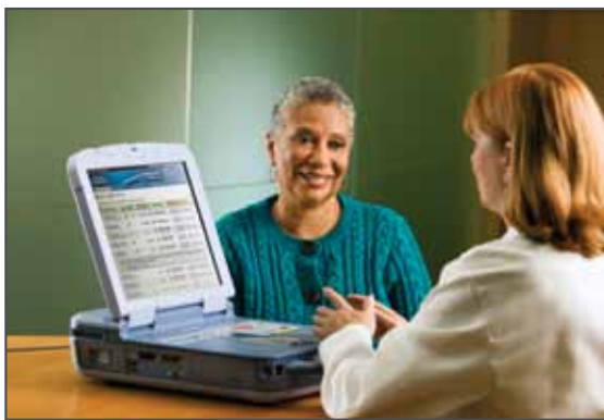
Doctors and nurses use a programmer to check an ICD and to communicate with it.
