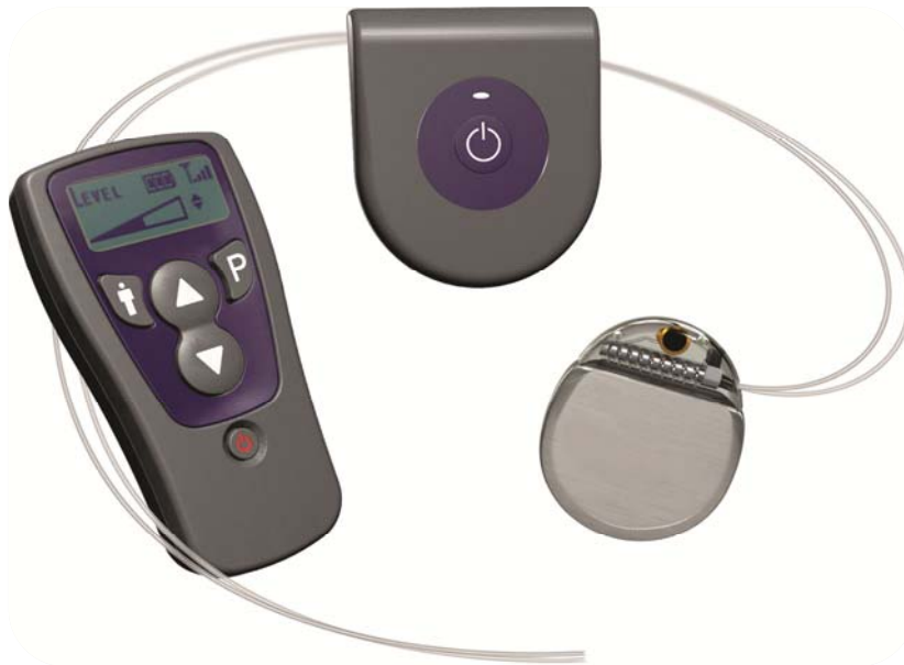
FROM LEFT TO RIGHT, THE PRECISION™ PLUS SPINAL CORD SYSTEM CONSISTS OF A REMOTE CONTROL, A CHARGER, AND AN IMPLANTABLE PULSE GENERATOR (IPG).
