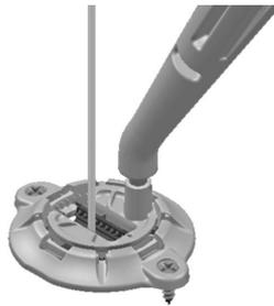
4. Push the Retaining Clip down into the Base. Make sure that the Retaining Clip is completely seated in the Base.
