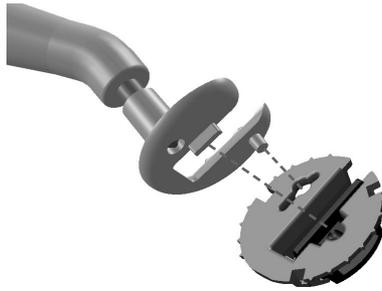
The post and the tab on the horseshoe end of the Placement/Removal tool line up with the clip release hole and closure dimple.
