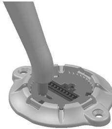
6. Gently push the Placement/Removal Tool partially toward the Slider and upward until the Retaining Clip releases from the Base.
