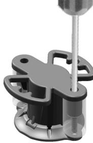
2. Using the Screwdriver gently push the Bone Screws through the Silicone Sleeve.
