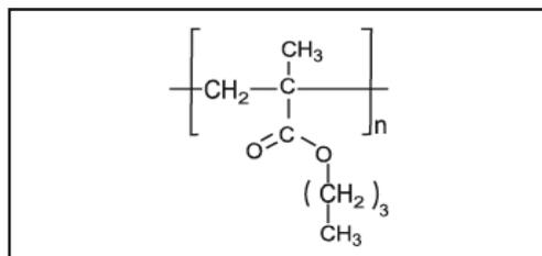
**Figure 2.2. The Chemical Structure of PBMA**
