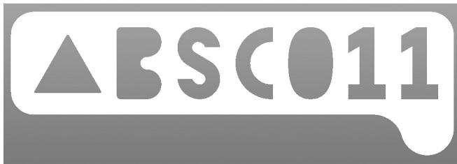
Figure 1-1. X-ray identifier for ADVANTIO MRI, INGENIO MRI, VITALIO MRI, and FORMIO MRI
