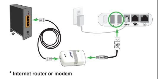
Keep your connection method plugged into the Communicator at all times.
