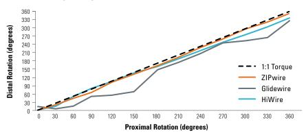
ZIPwire Guidewire better approaches a 1:1 torque response, while the Glidewire and HiWire Guidewires have a propensity to whip.
