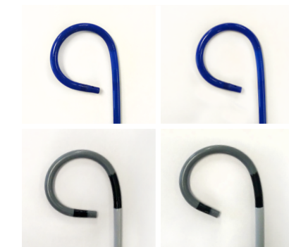
Figure 4. Tip curvature (photographs) Before fatigue conditioning (cycle 0) After fatigue conditioning and 20 steering cycles
