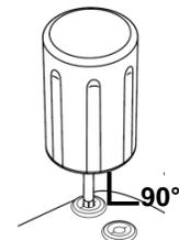
**NOTE:** Failure to properly insert the torque wrench in the pre-slit depression of the seal plug may result in damage to the plug and its sealing properties. Do not implant the device if any seal plugs appear to be damaged.
