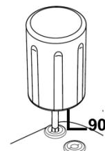
**STEP 6:** Remove the wrench by pulling it straight out of the connector block, maintaining a 90° angle
