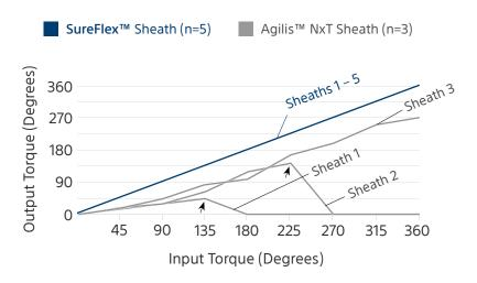
**Figure 3.** Individual sheath torque transfer (axial rotation) performance (arrows indicate sheath breakage)
