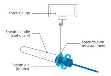
Figure 2. Tip deflection and dial tactile feedback test set-up
