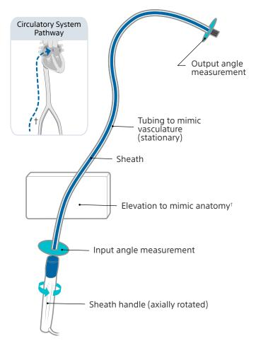
Figure 1. Axial rotation test setup
