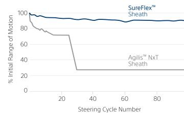
Figure 5. Percent of initial range-of-motion retained over 100 steering cycles with dilator and needle
