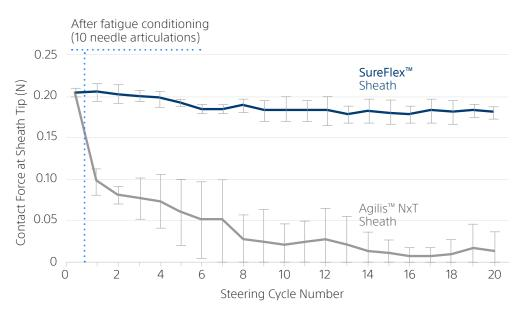
Figure 3. Average contact force over sheath steering cycles (data points are the mean ± standard error for 5 **SureFlex**<sup>™</sup> and 3 Agilis<sup>™</sup> NxT sheaths)
