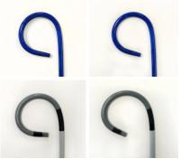
Before fatigue After fatigue conditioning (cycle 0)
