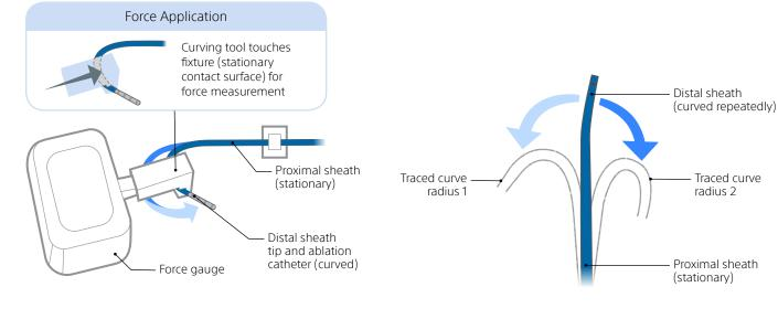
Figure 1. Contact force experimental setup
