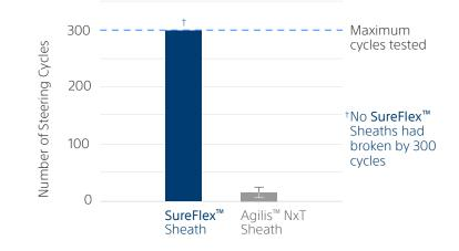
Figure 6. Number of cycles to failure (data are the mean ± standard error for 5 SureFlex<sup>™</sup> Sheaths and 6 Agilis<sup>™</sup> Sheaths)
