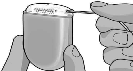
**CAUTION:** Verify proper DBS Extension insertion by checking impedances before tightening the Setscrew. Tightening the Setscrew down onto a contact can damage the DBS Extension.
