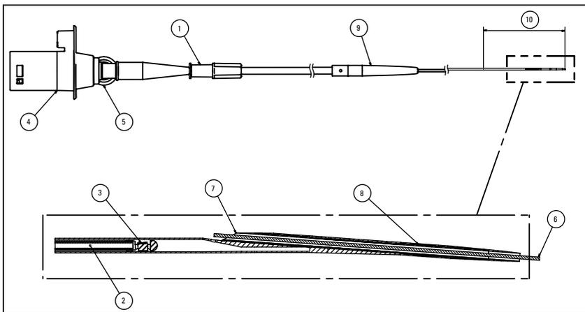
Figure 1. OptiCross™ 6 (40 MHz Coronary Imaging Catheter)
