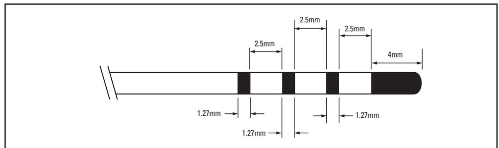
Figure 2. The Distal Segment of the Chilli II Catheter
