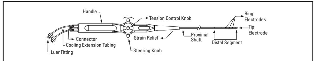
Figure 1. The Chilli II Catheter
