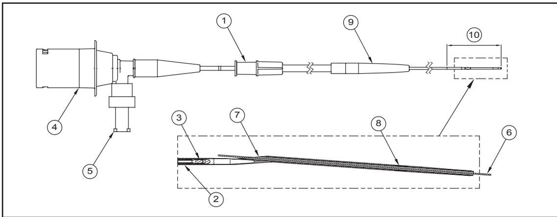
Figure 1. OptiCross™ 40 MHz Coronary Imaging Catheter
