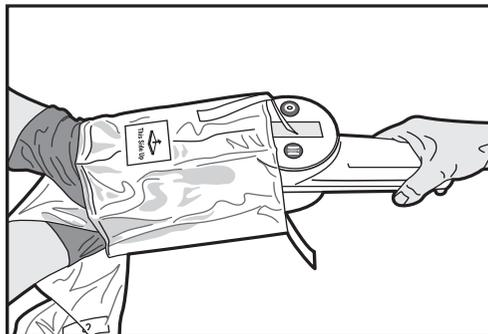
Figure 4. Inserting the MDU5 PLUS
