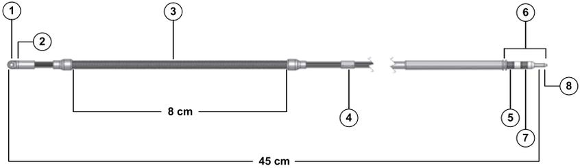
[1] Anchoring Hole, [2] Distal Sensing Electrode, [3] Defibrillation Coil, [4] Proximal Sensing Electrode, [5] Terminal electrode connection for proximal sensing electrode, [6] SQ-1 S-ICD connector (non-standard), [7] Terminal electrode connection for defibrillation coil, [8] Terminal Pin (electrode connection for distal sensing electrode)
