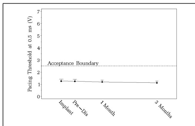
**Figure 1. ACUITY Steerable lead pacing thresholds with device in the programmed configuration. All patients implanted; N=101 (Mean, 95% confidence bound).**
