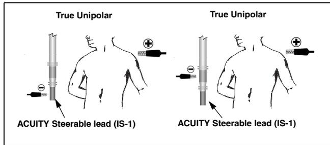
**Figure 20. LV Pacing Unipolar: Pacing system analyzer connections.**
