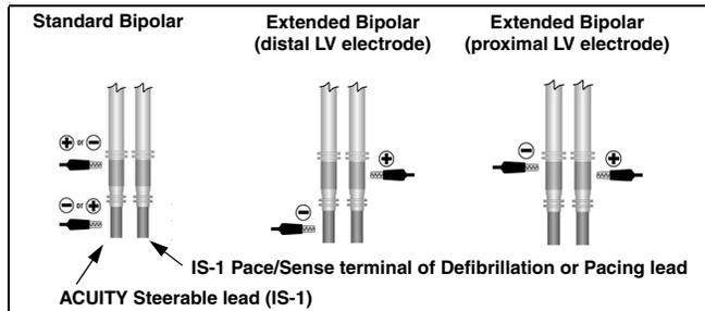
**Figure 21. LV Sensing: Pacing system analyzer connections.**
