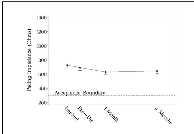
**Figure 3. ACUITY Steerable lead pacing impedances with device in programmed configuration. All patients implanted; N=101 (Mean, 95% confidence bound)**
