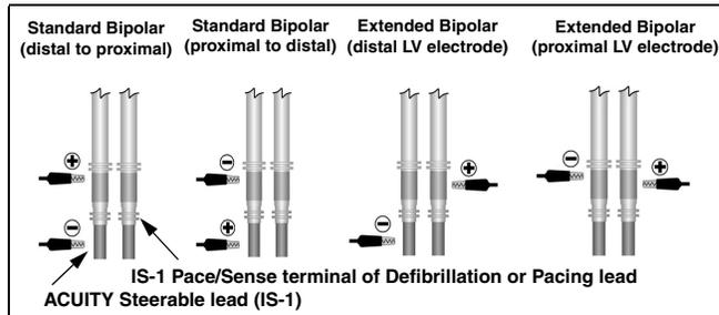
**Figure 19. LV Pacing Bipolar: Pacing system analyzer connections.**
