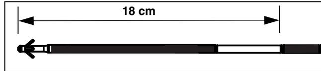
**Figure 2. Electrode spacing for the ENDOTAK RELIANCE lead is measured from the distal tip to the distal end of the proximal coil Electrode.**
