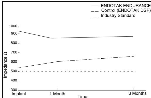
**Figure 1. ENDOTAK ENDURANCE Rx lead impedance by follow-up period. (n=98)**
