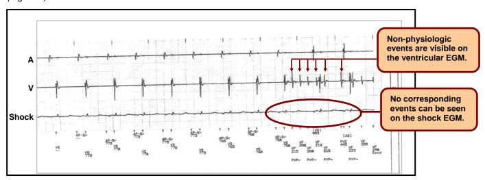
Figure 1. EGM indicating non-physiologic oversensing due to air bubbles escaping header through seal plugs.
