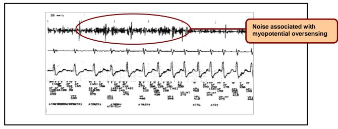
Figure 2. Example of oversensing of pectoral muscle activity due to significant atrial seal plug damage.
