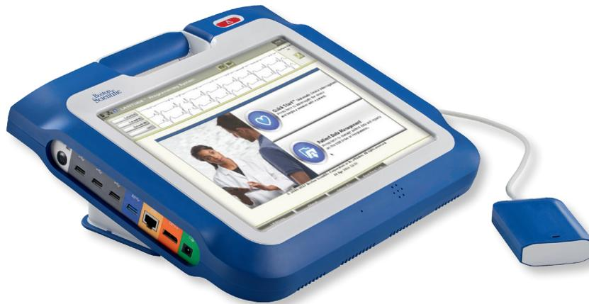
The Model 3300 Programmer is a portable cardiac rhythm management (CRM) programming system designed to allow health care providers to interrogate, monitor and program Boston Scientific implantable pulse generators (PGs).
