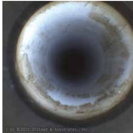
Inside a colonoscope suction/biopsy channel showing scratches and brown staining
