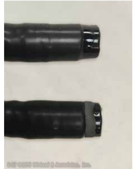
Distal ends of two gastroscopes (top one intact; bottom one damaged)
