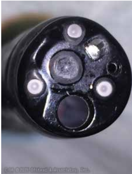
Distal tip of a colonoscope with a scratched and cloudy lens
