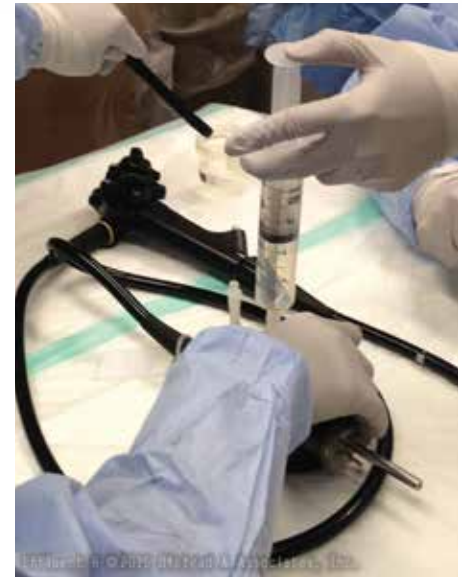
Two technicians conducting an ATP test of a colonoscope biopsy port
