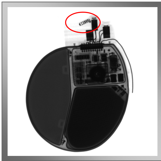
TELIGEN™ ICD and COGNIS™ CRT-D Uses Programmer Software Application: Model 2868/3868 X-ray Identifier: BOS112
