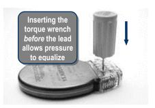
**NOTE:** Failure to properly insert the torque wrench in the pre-slit depression of the seal plug may result in damage to the plug and its sealing properties. Do not implant the pulse generator if the seal plugs appear to be damaged.
