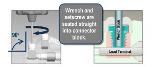
**Remove wrench.** Remove the torque wrench by pulling it straight out of the connecter block.
