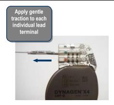
**Evaluate Lead Signals.** Evaluate the electrical performance of each lead after connecting to the pulse generator to provide final confirmation of a proper connection. Ensure the baseline atrial and RV/LV channels are free of artifacts. An improper connection could result in loss of therapy or inappropriate therapy.
