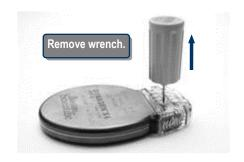
**Verify lead is secure.** Apply gentle traction to the lead to ensure a secure connection. If the lead terminal is not secure, reinsert the torque wrench as described above, and loosen the setscrew by slowly turning the wrench counterclockwise, until the lead is loose. Then repeat the steps above.
