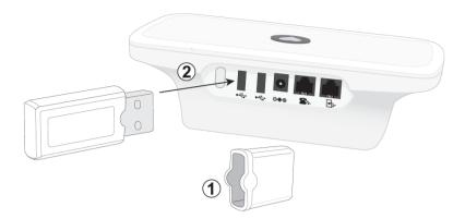
Figure 1. Connecting the LATITUDE USB Accessory Adapter
