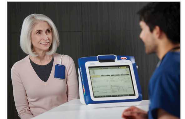
Doctors and health care providers use a programmer to check a pacemaker and communicate with it.
